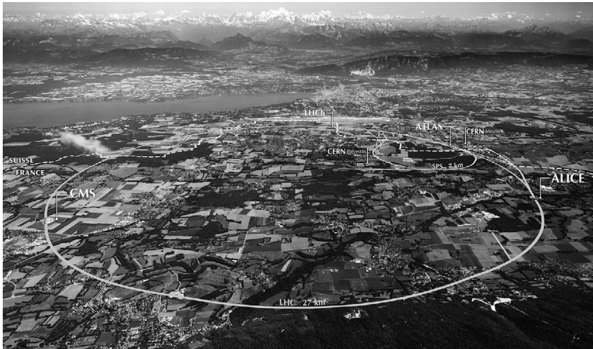
Figure 1: The circle represents the Large Hadron Collider (LHC), one of the most complex and ambitious scientific experiment yet built. It has a circumference of some 26 km. The proposed Future Circular Collider at CERN, if built, will have a circumference of 100 km. Image by Maximilien Brice (CERN) – CERN Document Server, CC BY-SA 3.0, https://commons.wikimedia.org/w/index.php?curid=29027732 .
